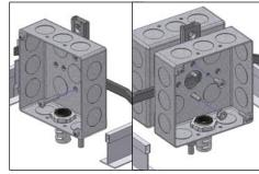
5A. For dual feeds, hang first J-box with long screw on bracket A. Take center knock-out on the second J-box. Screw second J-box to bracket B. Then add nut to connect two boxes together.
