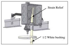
Insert feed cord into J-Box through bushing and canopy. Attach strain relief on the cord.
