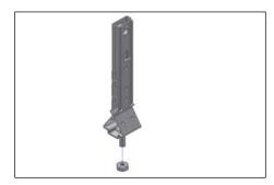
Insert bolt into Bracket A. Hook Bracket B onto Bracket A. Secure with nut (DO NOT TIGHTEN).
