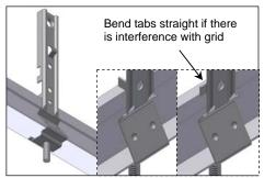
Insert bolt into bottom hole of Bracket A. then hook Bracket A onto grid.
