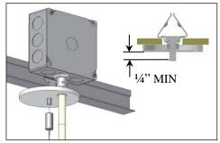
Place canopy flush with ceiling tile. Thread cable retainer onto bolt no less than 1/4".
