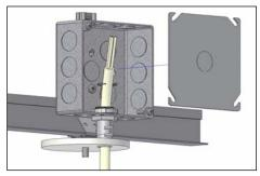
Connect wires and install the cover to J-Box with screws.
