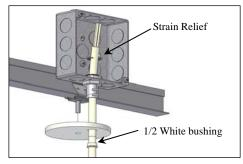
Insert feed cord into J-Box through bushings and canopy. Attach strain relief on the cord.
