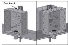
5. Hang J-Box assembly on bracket 5A. For dual feeds, hang first J-box with long screw on the bracket A. Take center knock-out on the second J-box. Screw second Jbox to bracket B. Then add nut to connect two boxes together.
