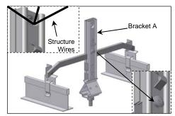
Adjust brackets to proper location then screw the brackets from A to B together. Secure the brackets to the structure above.
