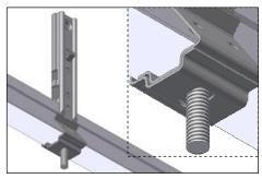
2. Hook Bracket B onto Bracket A
