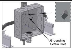
Hang J-Box on bracket A tab. For single feed, screw J-Box to brackets.
