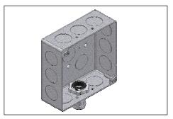
Attach black bushing and conduit fitting to J-box.
