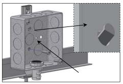
A tab. For single feed, screw J-Box to brackets.
