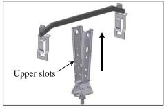
2. Slide hanger onto Caddy Bar and 3. fit Caddy Bar into upper slots in bracket.
