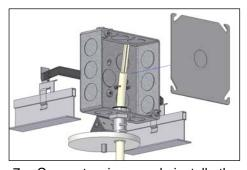
7. Connect wires and install the cover to J-Box with screws.
